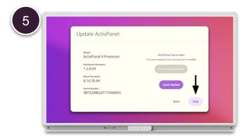
If your ActivPanel is connected has Internet connection. an automatic search for firmware updates is performed and you can choose to install the latest version or press Skip.
