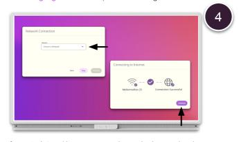
If your ActivPanel is not connected to a wired network, select Network settings to connect to a wireless network, or select Skip and do this later.
