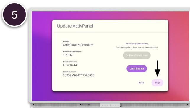
If your ActivPanel is connected has Internet connection. an automatic search for firmware updates is performed and you can choose to **install the latest version** or press **Skip**.
