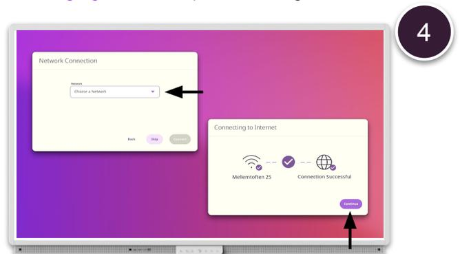
If your ActivPanel is not connected to a wired network, select **Network settings** to connect to a wireless network, or select **Skip** and do this later.
